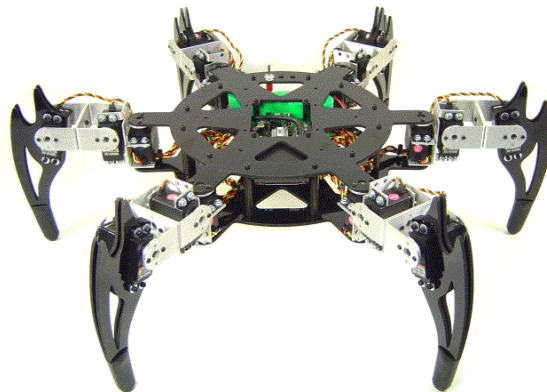
Figure 4. This figure shows a hexapod robot similar to the one that will be used to kick balls away from the fence. Hexapods are statically stable on three legs, meaning that they do not have to actively balance and they can use one or more legs to kick the tennis balls away from the fence.
